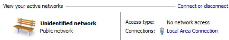
Illustration 2: Planet network displayed as Unidentified due to failure to obtain IP address.
