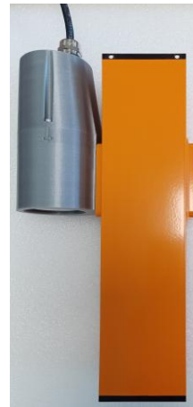
Figure 4. Connecting to the ROW using sunshield
